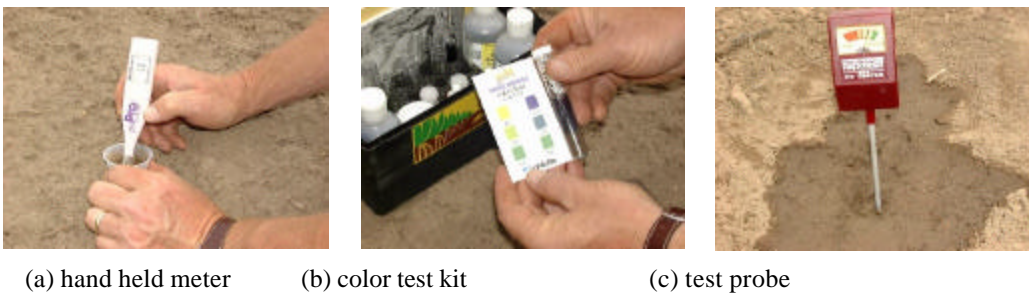
Figure 1. Three methods of measuring soil pH in the field.
