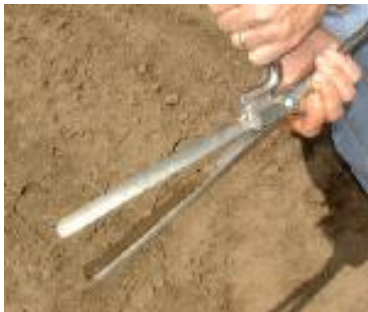
Fig. 2a Split tube design with M&amp;M probe
