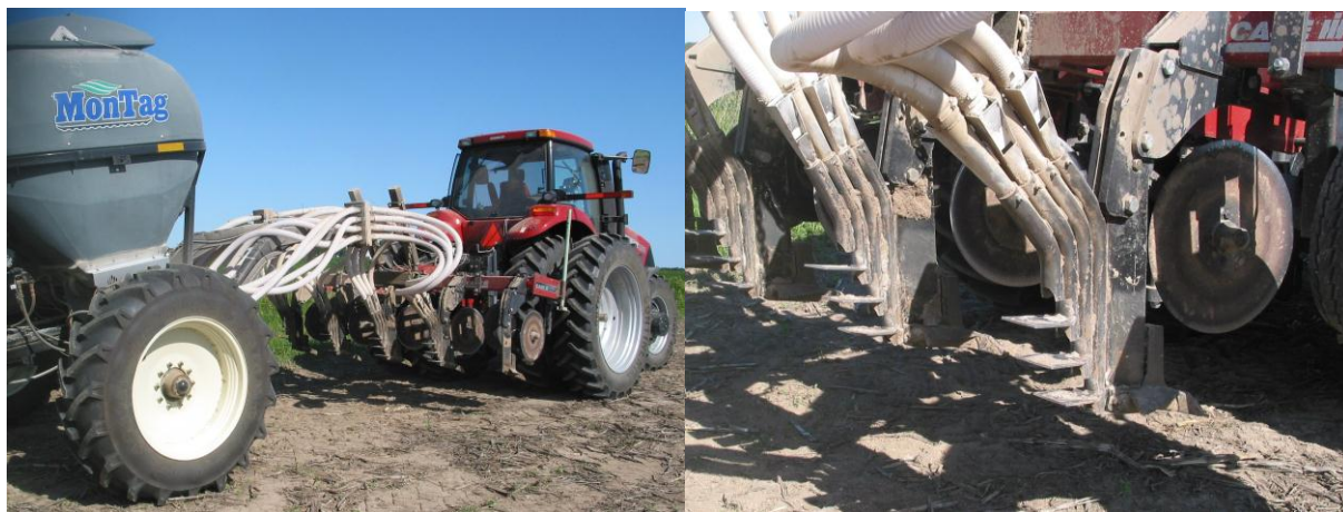
Figure 1. Deep placement applicator with Montag dry fertilizer air delivery system (left) and custom built applicator shank (right).
