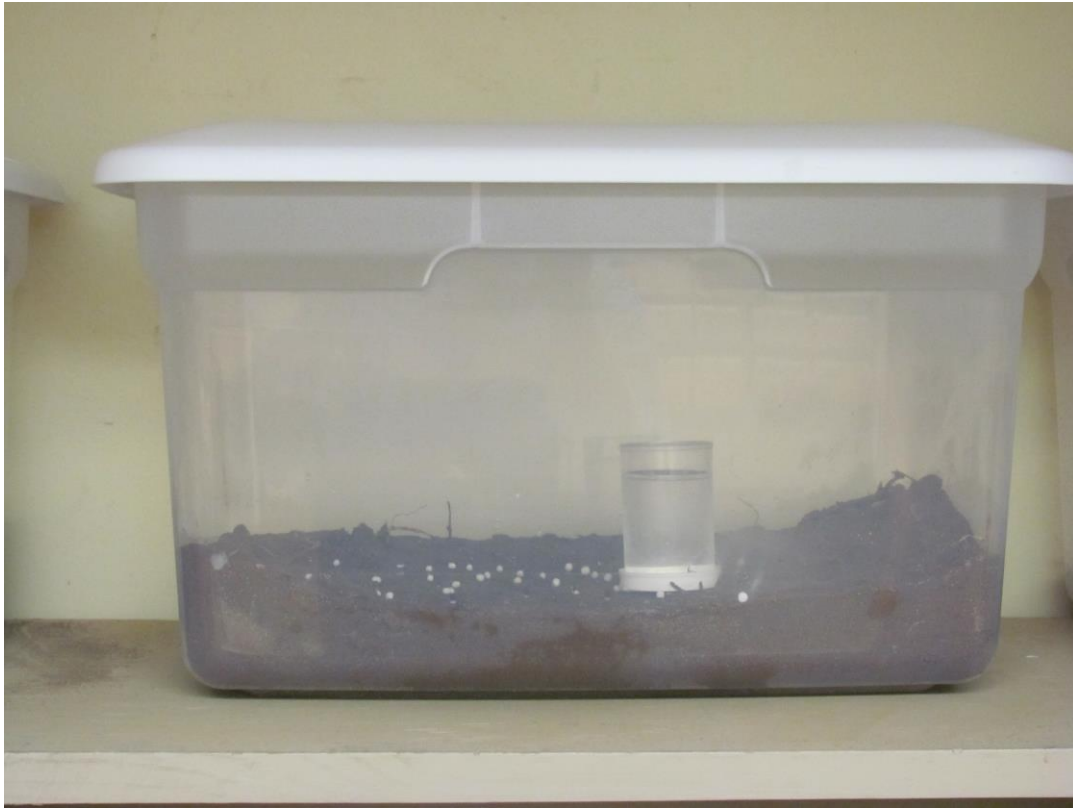
Figure 1. Chamber used for measuring ammonia volatilization with 2 dram vial serving as acid trap, note granular urea on soil surface
