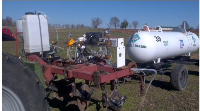
Figure 2. Cold flow unit, flow meter, and control valve used to apply anhydrous ammonia treatments.
